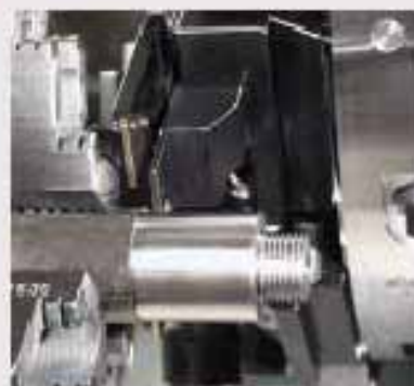
PULLEX' extremely compact design allows cut-off very close to the chuck jaws.
